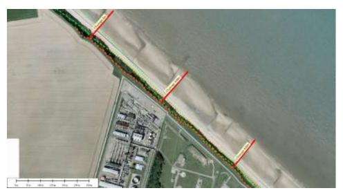
Figure 9.16 - The eastern end of the Bacton Gas Terminals frontage in 2009 with cliff top and toe positions mapped for 1946, 1992 and 2009 (red lines indicate chainage points marking the distance along the coast)
