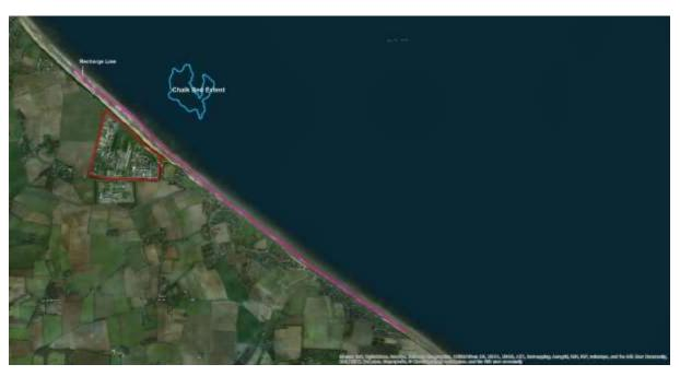
Figure 6-35. Line of placement (shown in pink along the Bacton to Walcott coast with Bacton Gas Terminals indicated within the red polygon and the extent of the chalk bed shown in blue)
