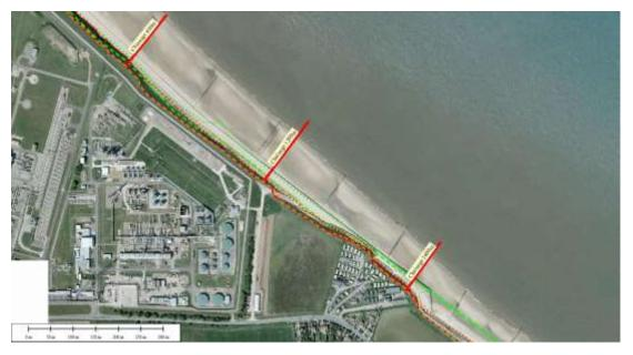
Figure 9.17 - The western end of the Bacton Gas Terminals frontage in 2009 with cliff top and toe positions mapped for 1946, 1992 and 2009
